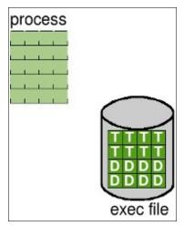
the size of the virtual space is mainly determined by the text (T) and data (D) pages in the executable file, with a few additional pages for the process' stack.
